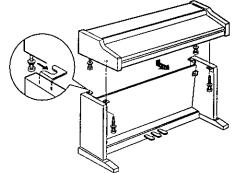
(1) Insert 2 black screws (A) in the 2 rear screw holes on the underside of the piano body, and turn each screw 5 or 6 times. Push the piano body forward so that the screws are fully inserted in the cutout of the metal piece on either side plank. (This enables you to easily position the piano body on the stand.) (2) Adjust the piano body so that the right and left sides project evenly over the stand.
