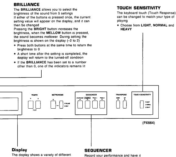
The display shows a variety of different setting values, and also the SEQUENCER and METRONOME tempos
