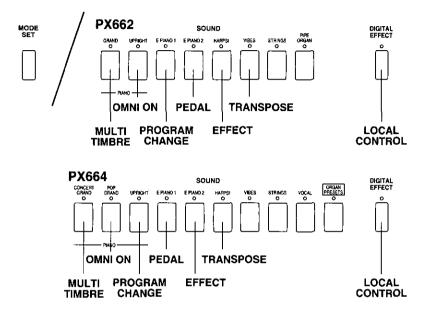
While the MODE SET button is depressed, the keyboard keys do not produce sound
